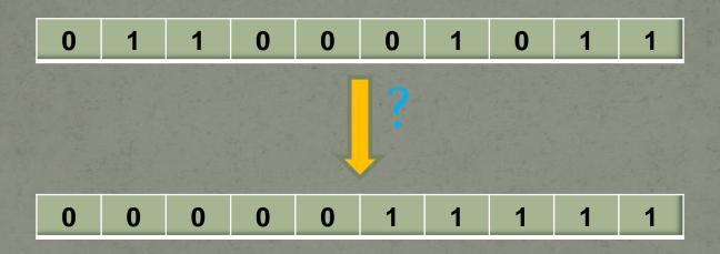
Problem: find algorithm which can be used to sort random data containing only 0 and 1(we want to get all 0 on the left and 1 on the right side of the series):
