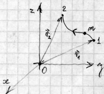
$$W_{12} \equiv \int_1^2 \vec{F} \cdot d\vec{r}, \quad \text{in general } W_{12} \text{ depends on path between points 1 and 2;}$$
